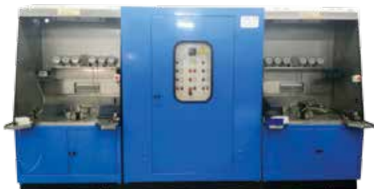
HPU valves test bench
