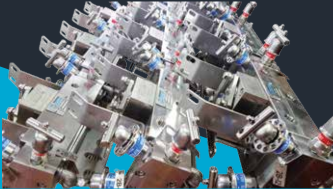
High pressure gas systems safety relief valve (Project ORMEN LANGE)
